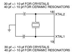
The oscillator, in any case, drives the internal clock generator. The clock generator provides the internal clocking signals to the chip. The internal clocking signals are at half the oscillator frequency, and define the internal phases, states, and machine cycles, which are described in the next section.
