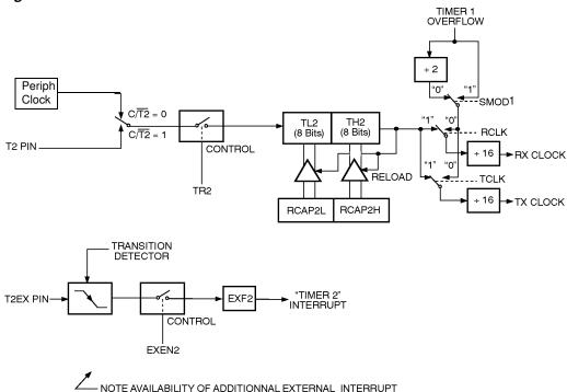
The baud rate generator mode is similar to the auto-reload mode, in that a rollover in TH2 causes the Timer 2 registers to be reloaded with the 16-bit value in registers RCAP2H and RCAP2L, which are preset by software.
