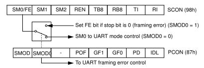
When this feature is enabled, the receiver checks each incoming data frame for a valid stop bit. An invalid stop bit may result from noise on the serial lines or from simultaneous transmission by two CPUs. If a valid stop bit is not found, the Framing Error bit (FE) in SCON register (see Table 2-17) bit is set.
