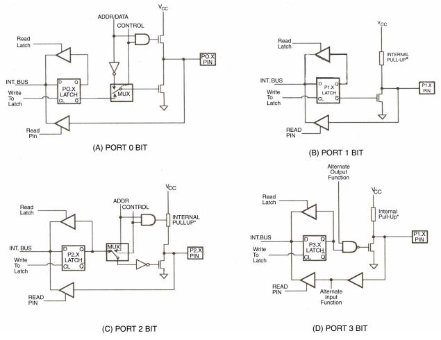
As shown in Figure 2-4, the output drivers of Ports 0 and 2 are switchable to an internal ADDR and ADDR/DATA bus by an internal CONTROL signal for use in external memory accesses. During external memory accesses, the P2 SFR remains unchanged, but the P0 SFR gets 1s written to it.
