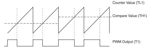
Figure 16-2. Timer 0/1 Pulse Width Modulation Mode
