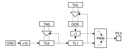
TL0 counts once every machine cycle (1 machine cycle = 12 clocks in X1 mode) and TH0 is the reload value for when TL0 overflows. Every time TL0 overflows TL1 increments by one, with TL0 overflowing after counting 256 minus TH0 machine cycles.
