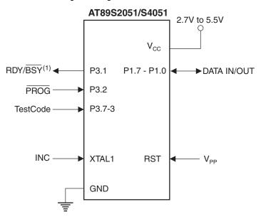
Sampling of pin P3.1 (RDY/BSY) is optional. In Parallel Mode, P3.1 will be pulled low while the device is busy. However, it requires an external passive pull-up to V<sub>CC</sub>. Also, note that P3.6 does not exist, so TestCode connects to P3.7, P3.5, P3.4, and P3.3.
