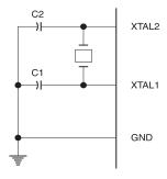
Note: C1, C2 = 5 pF  $\pm$ 5 pF for Crystals = 5 pF  $\pm$ 5 pF for Ceramic Resonators
