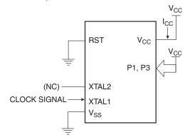
50. Clock Signal Waveform for  $I_{\text{CC}}$  Tests in Active and Idle Modes,
