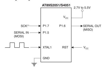
Note: 1. SCK frequency should be less than (XTAL frequency)/8.
